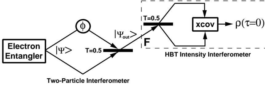
*Figure 3.* Proposed electron bunching and anti-bunching experiment. A two-electron entangler emits electrons in the spin-singlet state into a two-particle interferometer. A phase shift,  $\phi$ , is applied to spin down electrons in the upper arm. The output Fano factor after collision is measured using an HBT-type intensity interferometer.
