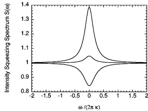
FIG. 10. Intensity squeezing spectrum outside the cavity for (from top to bottom)  $\eta=0.86$ ,  $0.87$ , and  $0.89$ , which correspond to  $g/(2\pi)=47.7$ ,  $50.9$ , and  $55.7$  MHz, respectively. The photon damping rate  $\kappa$  is 4 MHz, the decay in nonlasing modes  $R_{AB}=1500$  MHz, and  $R_{BC}=R_{CA}=10^4$  MHz. The frequency  $\omega/(2\pi)$  is normalized to  $\kappa$ .
