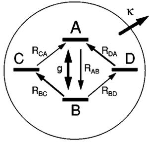
FIG. 2. Schematic level diagram of SQDL laser levels. The four levels are connected via rates  $R_{BC}$ ,  $R_{DA}$ ,  $R_{BD}$ , and  $R_{CA}$  (electron and hole tunneling). Spontaneous emission into nonlasing modes is described by the rate  $R_{AB}$ ;  $g$  is the QD-field coupling constant; and  $\kappa$  is the photon damping rate.
