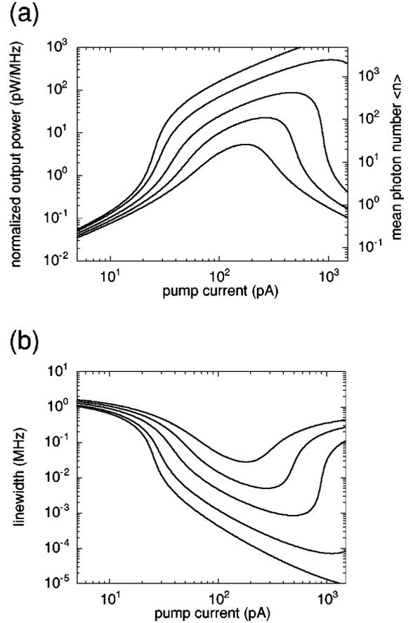
FIG. 6. Semiclassical approximation for (a) the output power and (b) the linewidth for  $\kappa = 4, 3, 2, 1$ , and 0.5 MHz. In (a) the output power is normalized to  $\kappa$ .
