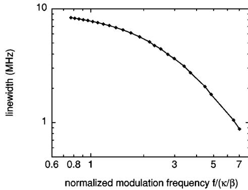
FIG. 9. Dependence of the linewidth on the driving frequency  $f$ .  $f$  is normalized to  $\kappa/\beta$ .
