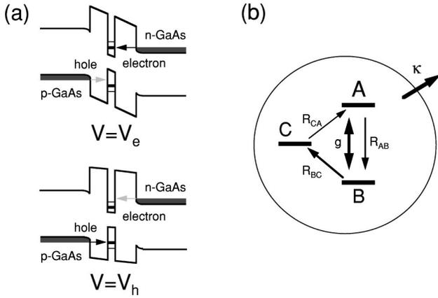
FIG. 7. (a) Schematic energy-band structure of the double-heterojunction resonant-tunneling structure when the resonant-tunneling condition is satisfied for electrons and holes at different bias voltages  $V = V_e$  and  $V = V_h$ . (b) Schematic level diagram of the SQDL laser in this situation. Periodic switching between  $V = V_e$  and  $V = V_h$  results in a periodic switching between the situations  $R_{BC} = 0$ ,  $R_{CA} \neq 0$  and  $R_{CA} = 0$ ,  $R_{BC} \neq 0$ .
