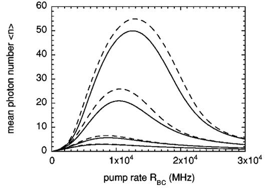
FIG. 3. Dependence of the mean photon number  $\langle n \rangle$  in the lasing mode on the pump rate for different photon damping rates  $\kappa$  (from bottom to top  $\kappa = 6, 5, 4, 3.5$  MHz), coupling strength  $g/(2\pi) = 31.8$  MHz, and relaxation rate  $R_{AB} = 1500$  MHz. Dashed curves are semiclassical approximations.
