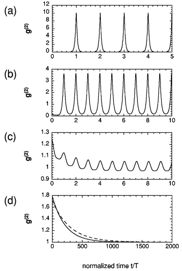
FIG. 8. Second-order correlation function  $g^{(2)}$  for different modulation frequencies  $f$ . (a)  $\beta f = 0.016\kappa$ , (b)  $\beta f = 0.05\kappa$ , (c)  $\beta f = 0.16\kappa$ , (d)  $\beta f = 1.6\kappa$ . For all curves  $\kappa = 5$  MHz,  $\beta = 0.016$ ,  $g/(2\pi) = 31.8$  MHz,  $R_{BC} = 10^4$  MHz, and  $R_{AB} = 1500$  MHz. The time is normalized to  $T = 1/f$ .
