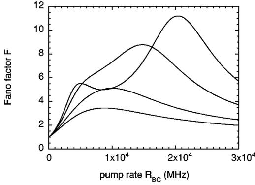
FIG. 4. Dependence of the Fano factor  $F$  on the pump rate for different photon damping rates  $\kappa$  (from bottom to top  $\kappa = 6, 5, 4, 3.5$  MHz), coupling strength  $g/(2\pi) = 31.8$  MHz, and relaxation rate  $R_{AB} = 1500$  MHz.
