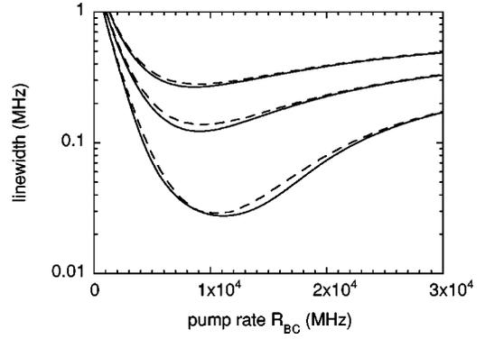
FIG. 5. Calculated linewidth of the SQDL when the pump rate is changed. From bottom to top:  $\kappa = 4, 5, 6$  MHz. The other parameters are the same as in Fig. 3. Dashed curves are semiclassical approximations.
