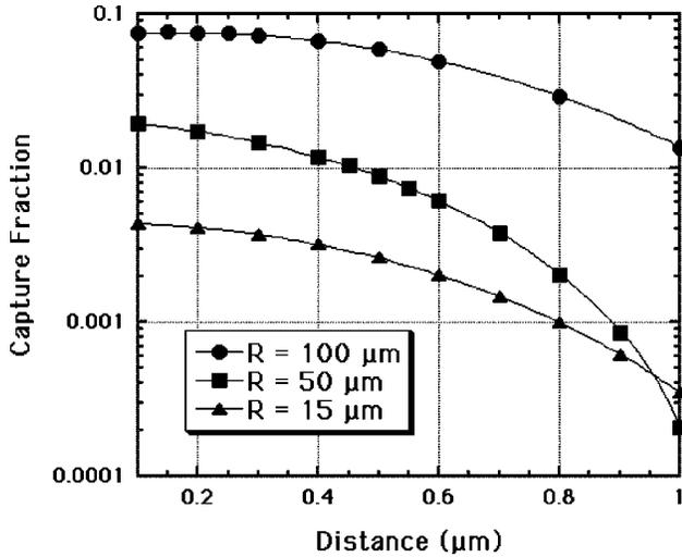
FIG. 2. Calculated capture fractions  $\beta$  for the laser with a single dot, as a function of the microsphere-sample distance.  $\beta$  is the fraction of spontaneous emission from the dot that is captured by the whispering-gallery mode of the sphere. Calculations are done for different sphere radii  $R$  assuming that the depth,  $D$ , of the dot in the sample is  $0.1 \mu\text{m}$ .
