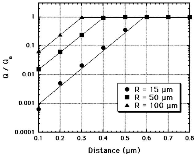
FIG. 3. Calculated quality factor  $Q$  of the whispering-gallery mode in a fused-silica microsphere as the sphere is brought towards a GaAs surface. Calculations are done for different sphere radii  $R$  as a function of sphere-sample distance. Results are normalized by the maximum quality factor  $Q_0$  of the mode, assumed to be  $5 \times 10^8$ .
