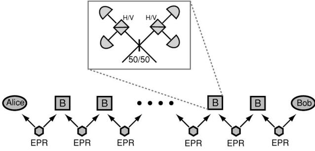
FIG. 3. Experimental setup for quantum key distribution with entanglement swaps.
