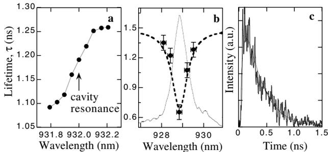
FIG. 3. Spontaneous emission lifetime and photoluminescence intensity vs wavelength for (a) a QD planar microcavity and (b) a QD post microcavity with a diameter of  $2.5 \mu\text{m}$ . In (c) the time-dependent spontaneous emission is shown for a single InAs QD, resonant with the fundamental mode of a  $0.5 \mu\text{m}$  diameter post microcavity.
