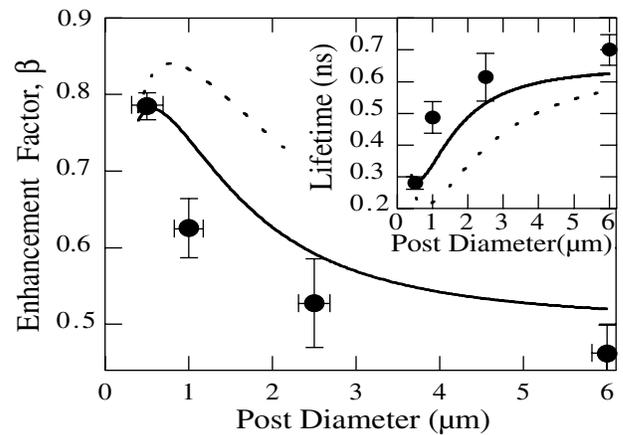
FIG. 4. Spontaneous emission coupling coefficient into the fundamental spatial mode,  $\beta$ , vs the post diameter.  $\beta$  for a single QD in the  $0.5 \mu\text{m}$  diameter post is 0.78. Solid lines indicate the calculated values. In the inset, the experimental and theoretical spontaneous emission lifetimes are plotted as a function of the post diameter. (Solid lines: an average over the post; dashed lines: a single dot at the post center.)
