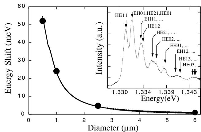
FIG. 2. Measured and calculated energy shifts of the fundamental cavity mode vs post microcavity diameter at 4 K. In the inset, the PL spectrum at 4 K from a  $5 \mu\text{m}$  diameter post microcavity is shown together with the predicted cavity mode eigenenergies (labeled according to transverse waveguide modes).
