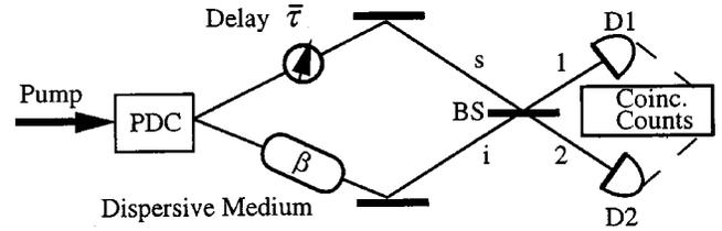
FIG. 3. A HOM interferometer with dispersive delay added to the lower arm. The pump beam (or pulse) creates signal ( $s$ ) and idler ( $i$ ) photons in the PDC that are later brought together at a beam splitter and counted in coincidence at detectors  $D1$  and  $D2$ .
