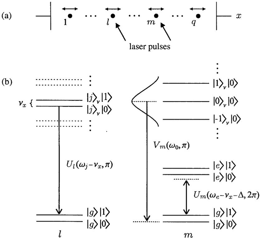
Figure 3. Phase-gate implementation. (a) Ion trap with pulses applied to ions  $l$  (control) and  $m$  (target). (b) Level scheme in each ion, with Rydberg levels  $j$  and auxiliary levels  $g$  and  $e$ . Three types of pulse are used:  $U_l(\omega_j - \nu_x, \pi)$ ,  $V_m(\omega_0, \pi)$  and  $U_m(\omega_e - \nu_x - \Delta, 2\pi)$ . See text for details.
