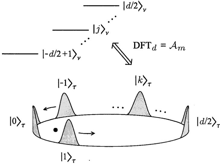
Figure 2. The Fourier conjugate of the energy-level basis  $|j\rangle_\nu$  consists of wave-packet states  $|k\rangle_\tau$  evenly distributed in time around a classical orbit. A radial wave-packet basis can be thought of as an ensemble of such orbits with different orientations for the ellipses.
