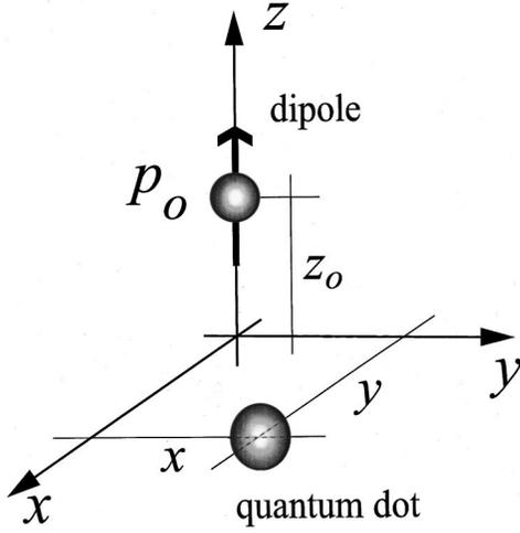
Fig. 4. Simplified configuration of a quantum dot ( $\mathbf{r} = x\mathbf{n}_x + y\mathbf{n}_y$ ) interacting with a laser-illuminated metal tip. The tip is replaced with a vertical dipole ( $\mathbf{r}_0 = z_0\mathbf{n}_z$ ) with moment  $p_0$  and oriented along the  $z$  axis.
