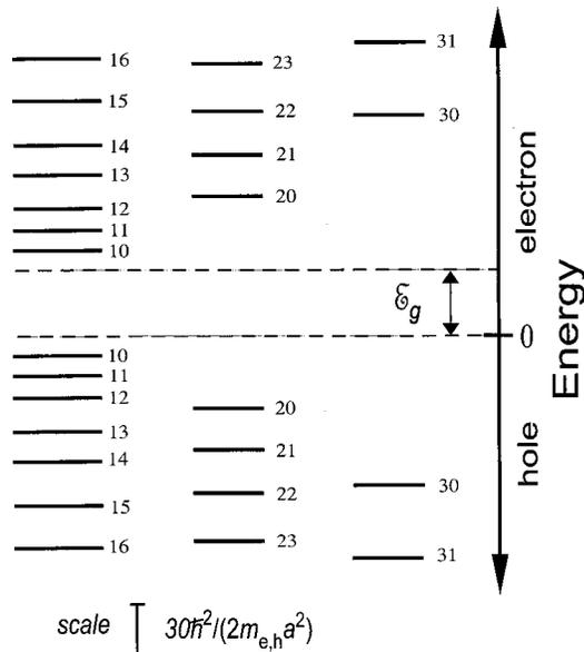
Fig. 1. Energy-level diagram of a spherical quantum dot according to Eqs. (14) and (15). Each energy level is characterized by quantum numbers  $n$  and  $l$ , and its degeneracy corresponds to quantum number  $m$ . Differently from the case of a hydrogen atom, quantum number  $n$  does not restrict the number of suborbitals  $l$ .
