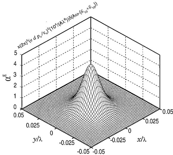
Fig. 6. Electric dipole absorption rate  $\langle \alpha^E \rangle$  as a function of normalized lateral coordinates ( $x/\lambda, y/\lambda$ ). The height of the excitation dipole is  $z_0 = 0.025\lambda$ .  $e, d$ , and  $p_0$  denote the elementary charge, the lattice constant, and the dipole moment, respectively.
