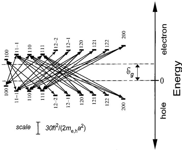
Fig. 2. Diagram of the allowed electric quadrupole transitions in a spherical quantum dot. The energy levels are labeled by the quantum numbers  $nlm$  (electron) and  $rst$  (hole). The selection rules are  $|l - s| = \pm 1$  and  $(m - t = \pm 1 \text{ or } m - t = 0)$ . The allowed electric quadrupole transitions exclude the allowed electric dipole transitions.
