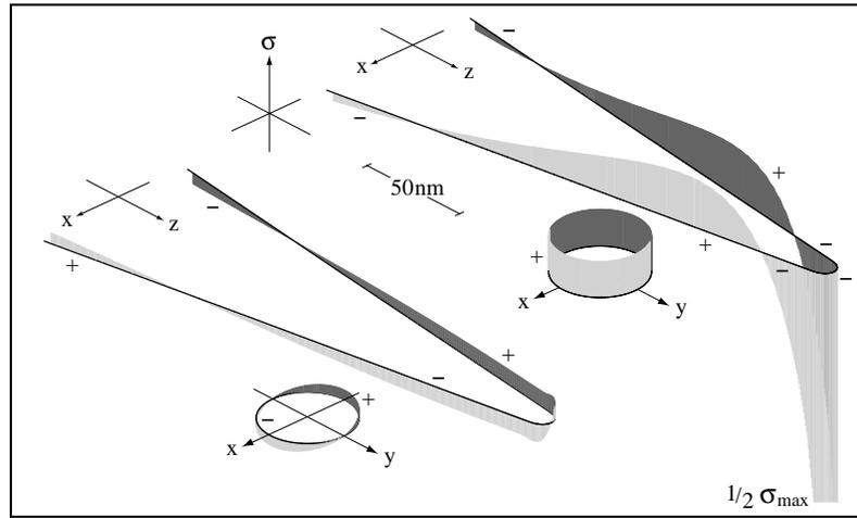
**Fig. 6.** Induced surface charge density corresponding to Fig. 5a (left) and Fig. 5b (right). The surface charges form a standing wave in each case. In Fig. 5a, the surface charge wave has a node at the end of the tip, whereas in Fig. 5b there is a large surface charge accumulation at the foremost part, responsible for the field enhancement.
