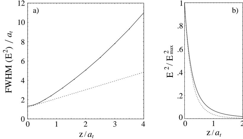
**Fig. 9.** Comparison of the nonretarded fields of a single dipole (dotted curves) and the rigorous solution for the laser illuminated metal tip (solid curves). Figure a) shows the lateral spread of the field (perpendicular to tip axis) as a function of the distance  $z$  from the foremost point of the tip. Figure b) shows the decay of the field along the tip axis. A normalization with the tip radius  $a_t = 5nm$  is applied.
