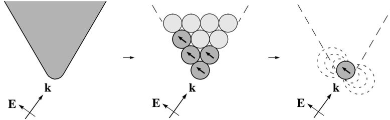
**Fig. 4.** Illustration of the coupled dipole approach. A macroscopic object is subdivided into individual microscopic dipolar subunits. Each dipole moment can be calculated self-consistently by using the Green's function formalism. In a rough approximation the field in front of a metal tip can be replaced by the field of a single dipole. However, the parameters of the polarizability have to be deduced from a rigorous calculation.
