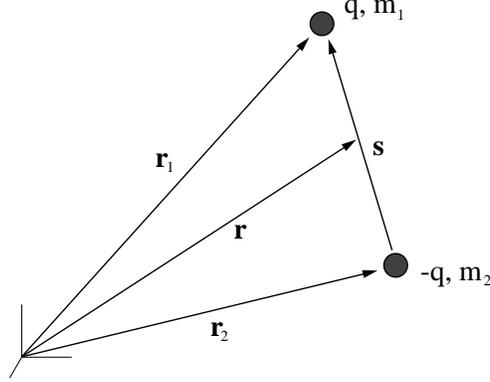
**Fig. 3.** Graphical representation of the symbols used to derive the mechanical force in the dipolar limit.  $\mathbf{r}$  denotes the center of mass coordinate. The two particles are bound to each other by the potential  $U$ .
