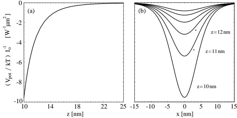
**Fig. 10.** Trapping potential  $V_{pot}$  along the tip axis (a) and along a transverse direction at  $z = a_t + a_p$  beneath the tip. An enhancement factor of  $f = 3000$  is assumed. The radii of tip and particle are  $a_t = a_p = 5 \text{ nm}$ . The dielectric constant of particle and environment are  $\varepsilon_p = 2.5$  (biomolecule) and  $\varepsilon_s = 1.77$  (water), respectively. Normalization with  $k_B T$  and incident intensity  $I_o$ .
