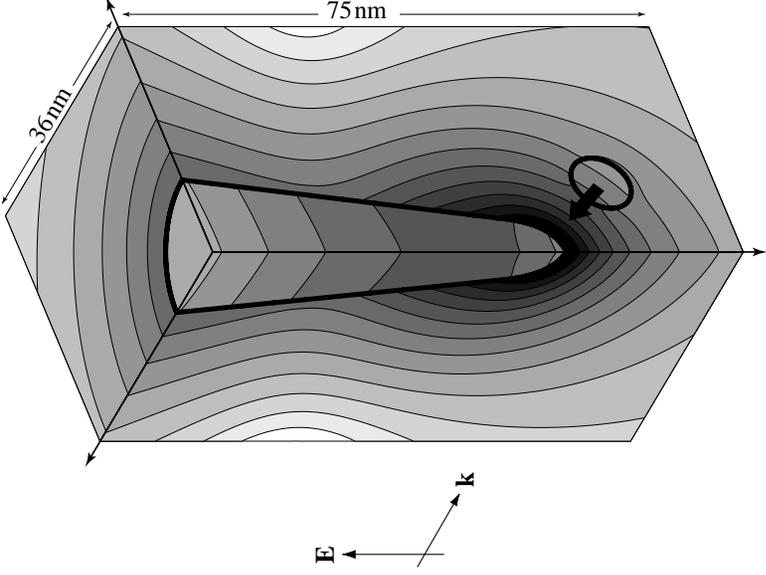
**Fig. 7.** Perturbation of the near-field by a particle being trapped ( $\epsilon = 2.5$ ,  $10\text{ nm}$  diameter). The field inside the particle is highly inhomogeneous, requiring rigorous calculation of the trapping force. The arrow indicates the direction of the trapping force. Same scaling as in Fig. 5b.
