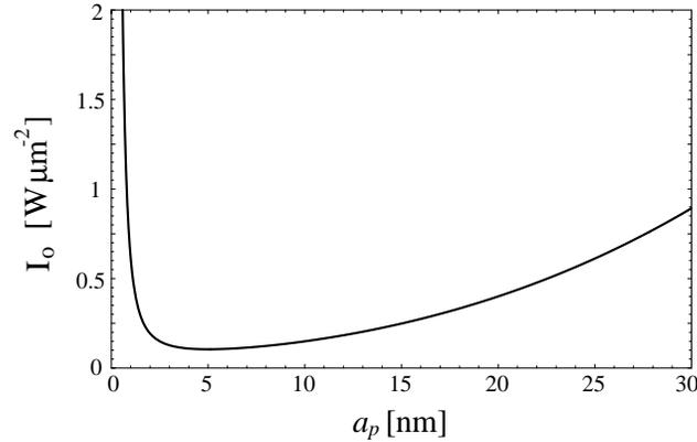
**Fig. 11.** Minimum trapping intensity  $I_o$  as a function of the particle radius  $a_p$ . An enhancement factor of  $f = 3000$  is assumed and the tip radius is  $a_t = 5 \text{ nm}$ . The dielectric constant of particle and environment are  $\epsilon_p = 2.5$  (biomolecule) and  $\epsilon_s = 1.77$  (water), respectively.
