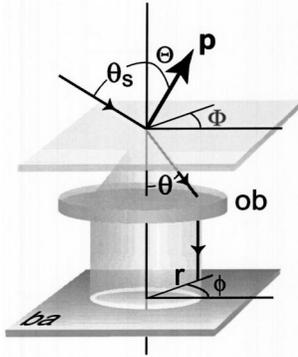
Fig. 1. Coordinate system used for calculations:  $\mathbf{p}$ , dipole moment; ob, the objective lens; ba, the back aperture of the objective lens.
