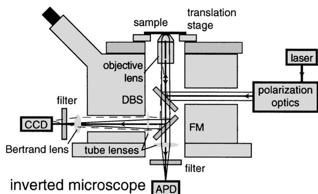
Fig. 3. Experimental setup consisting of an inverted microscope, a green excitation laser ( $\lambda = 532$  nm), a polarization optics box containing a half-wave plate, a quarter-wave plate, and a mode converter (see Ref. 29). DBS, dichroic mirror; FM, flip mirror; APD, avalanche photodiode; CCD, a cooled CCD camera.
