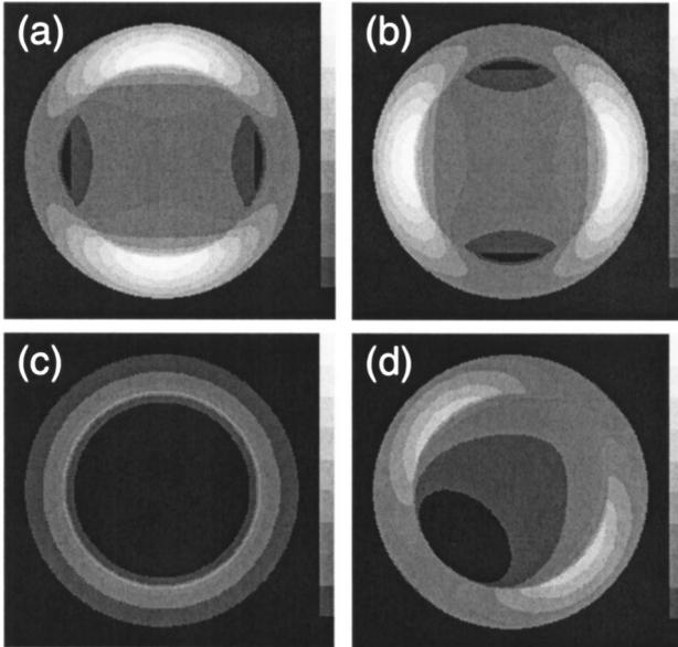
Fig. 2. Calculated emission patterns of a dipole at an air-glass interface ( $n_{\text{air}} = 1.0$ ,  $n_{\text{glass}} = 1.52$ ) in the back-aperture plane of a NA = 1.4 objective lens: (a)  $\Theta = 90^\circ$ ,  $\Phi = 0^\circ$  (horizontal dipole); (b)  $\Theta = 90^\circ$ ,  $\Phi = 90^\circ$  (horizontal dipole); (c)  $\Theta = 0^\circ$ ,  $\Phi = 0^\circ$  (vertical dipole); (d)  $\Theta = 45^\circ$ ,  $\Phi = 45^\circ$ .
