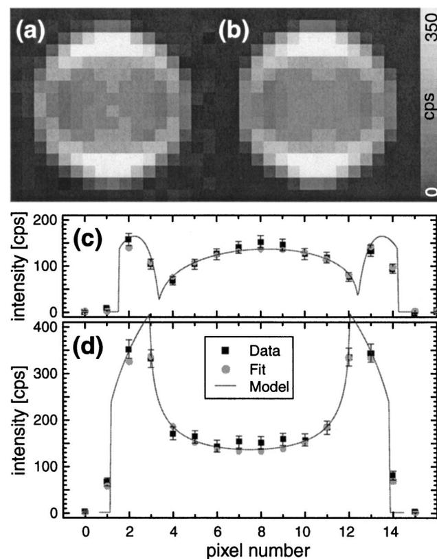
Fig. 4. Example of an observed emission pattern: (a) measured data; (b) fitted pattern; (c), (d), cross sections along a horizontal and a vertical line through the center of the pattern, respectively.
