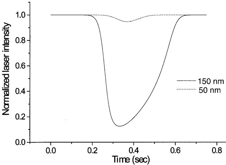
Figure 5. Calculated laser intensity for a 50 nm and a 150 nm particle passing exactly through the laser focus. The feedback loop automatically attenuates the laser intensity in order to prevent trapping of the larger particle.
