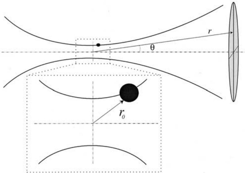
Figure 3. Illustration of the relative position of the detector and a particle near the laser focus. The parameters indicated in the figure are used in the derivation of equations (10)–(11). Because of the large distance between particle and detector the angle  $\theta$  is approximately the same for all particle positions near the laser focus.
