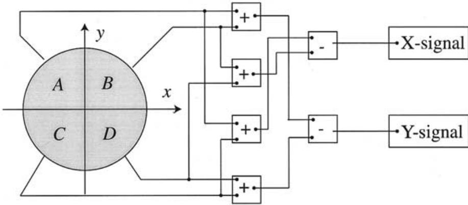
Figure 2. Computation of the differential signals  $\Delta x$  and  $\Delta y$  given the signals from the quadrant detector. The differential signal  $\Delta x$  represents a particle's motion along the flow channel ( $x$ -direction). The differential signal  $\Delta y$  represents a particle's motion transverse to the flow channel ( $y$ -direction).
