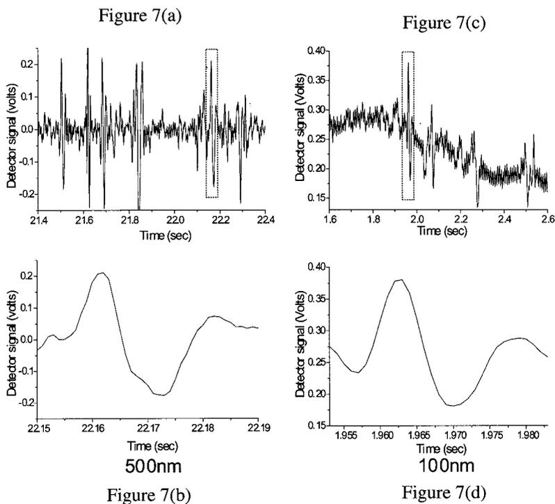
Figure 7. Experimental measurements of the quadrant detector signal for particles passing close to the focus. (a), (b) 500 nm particles trace; (c), (d) 100 nm particle trace. Dashed rectangles show magnified area. Notice asymmetry in (b) compared to (d).
