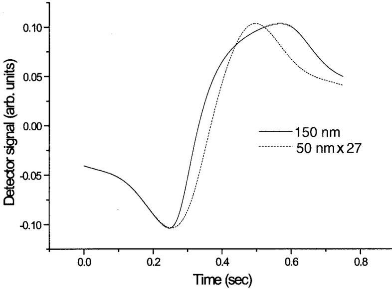
Figure 4. Calculated quadrant detector signal ( $\Delta x$ ) for a 50 nm and a 150 nm particle passing exactly through the laser focus. The two particles can be clearly distinguished based on the different time traces. Note that the time trace for the 50 nm particle is scaled by a factor of 27 in the amplitude. See text for details.
