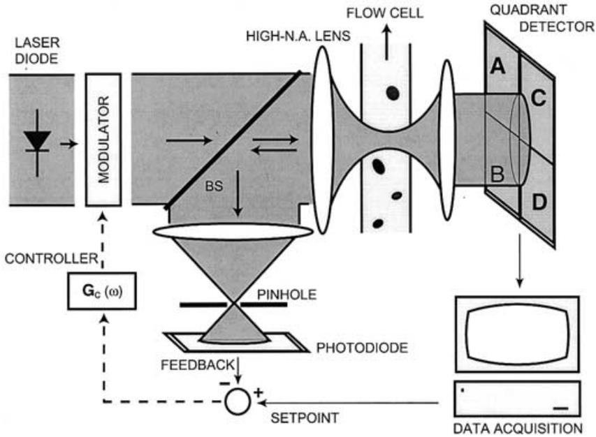
Figure 1. Illustration of the gradient-force nanoparticle detector. Light from a laser source is tightly focused into a flow cell. Particles moving in the flow cell are deflected from their original path due to the optical gradient force. The deflection is monitored by a quadrant detector located in transmission. A detector located in reflection is integrated into a feedback loop which prevents particles from being trapped by automatically attenuating the laser intensity.
