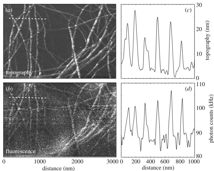
Figure 4. Simultaneous (a) topographic image and (b) near-field two-photon excited fluorescence image of J-aggregates of PIC dye in a PVS film on a glass substrate. Cross-sections along the dashed white lines indicate that the optical image (d) has slightly better resolution than the topographic image (c) (FWHM of 25 nm against 30 nm).
