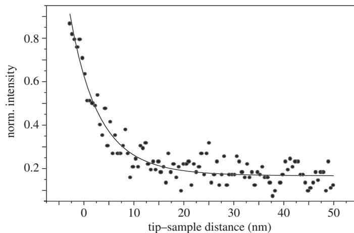
Figure 5. Distance dependence of the two-photon excited fluorescence from J-aggregates after femtosecond excitation at 833 nm.
