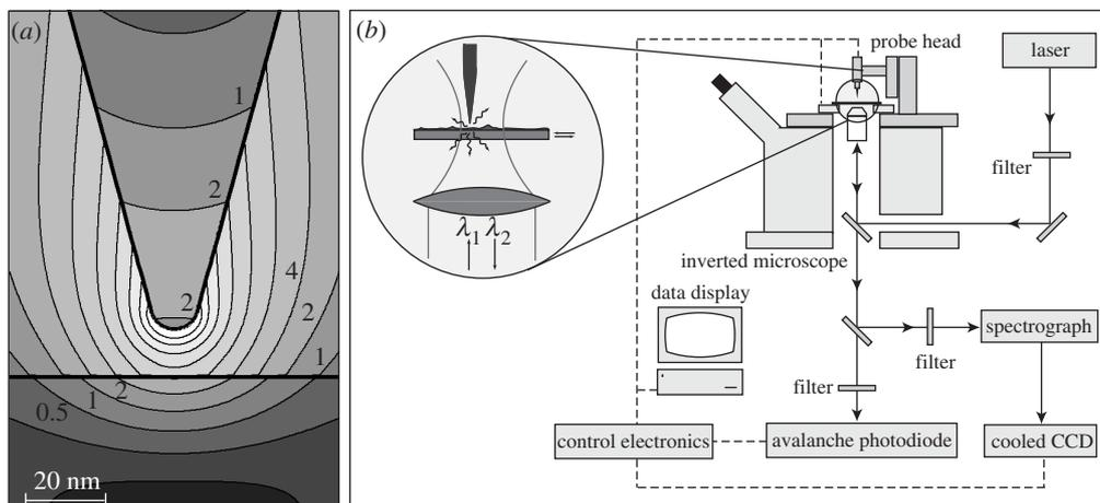
Figure 1. (a) Calculated field distribution  $[|E_{\text{local}}(\mathbf{r}, \omega)|^2]$  near a gold tip located above a glass substrate and irradiated by an on-axis focused Hermite Gaussian (1,0) laser mode. The contour lines scale by a factor of two. (b) Schematic of the experimental set-up. A sharp metal tip is scanned through a tightly focused laser beam. The optical signal is detected either by an APD or by a combination of spectrograph and a CCD.
