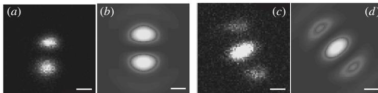
Figure 3. The intensity of the SH signal emitted by a gold tip which is raster scanned through the focus of (a) a Gaussian and (c) a Hermitian–Gaussian beam, respectively. Calculated distributions of the longitudinal fields in the focus of (b) a Gaussian and (d) a Hermitian–Gaussian beam, respectively. The scale bar is 250 nm.
