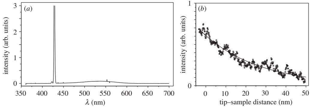
Figure 2. (a) Spectrum detected for a gold tip after fs-pulse excitation at 860 nm by the longitudinal field of a tightly focused Gaussian laser beam. A huge second-harmonic peak at 430 nm and a weak broadband continuum are observed. (b) Evolution of the second-harmonic intensity as a function of tip-sample separation (circles). The solid line represents an exponential fit with a decay length of 25 nm.
