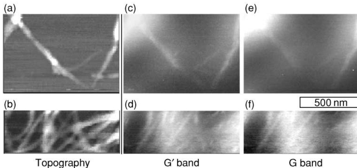
Fig. 5. (a and b) Topographic images of SWNT bundles (max. height 20 nm). (c–f) Raman images of the same area acquired by detecting the intensities of the Raman bands  $G'$  and  $G$  (cf. Fig. 2b). 50 ms integration time per pixel. All images have a width of 1  $\mu\text{m}$ .
