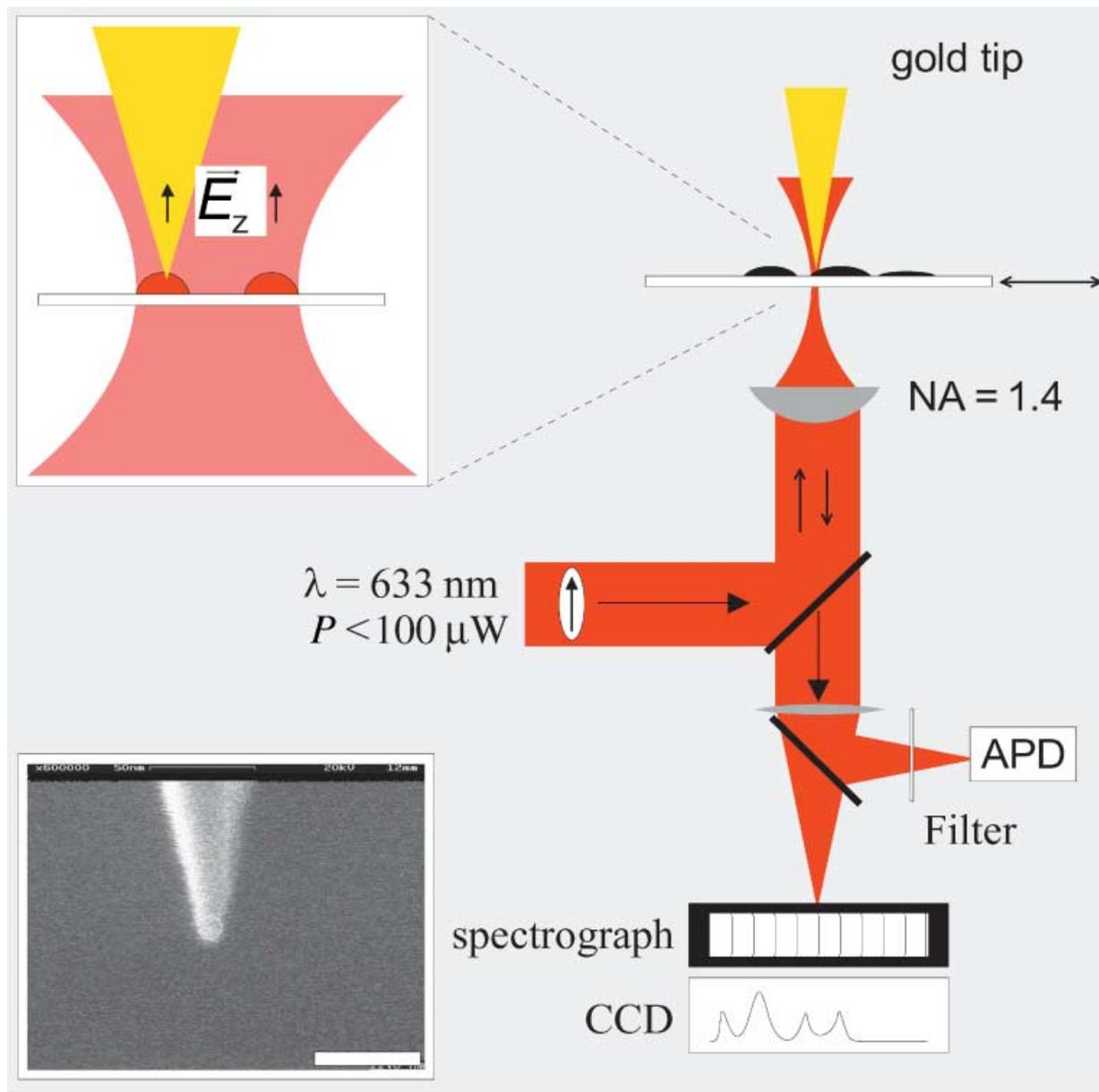
**Fig. 1.** Experimental set-up. (Inset upper left) Distribution of the longitudinal electric field  $\vec{E}_z$  within a tightly focused laser beam (schematic) (Sick *et al.*, 2000). (Inset lower left) Scanning electron micrograph of an ultra-sharp gold tip produced by electrochemical etching. Scale bar, 50 nm.
