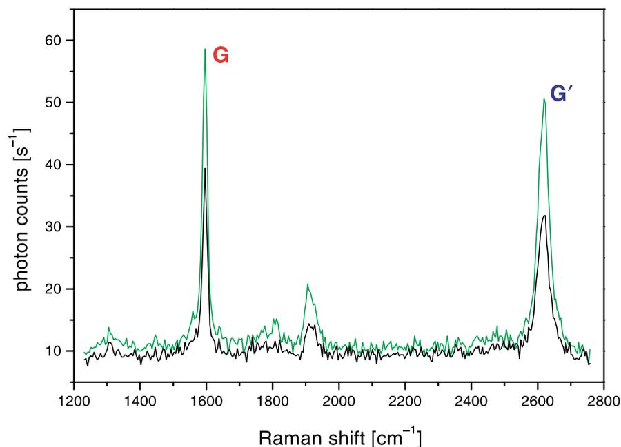
**Fig. 3.** Raman spectra detected with a sharp metal tip (green line) on top of the sample (distance  $\approx 1 \text{ nm}$ ) and with the tip retracted by  $2 \mu\text{m}$  (black line). Note, the intensities of all Raman bands are increased with the tip close to the SWNTs.
