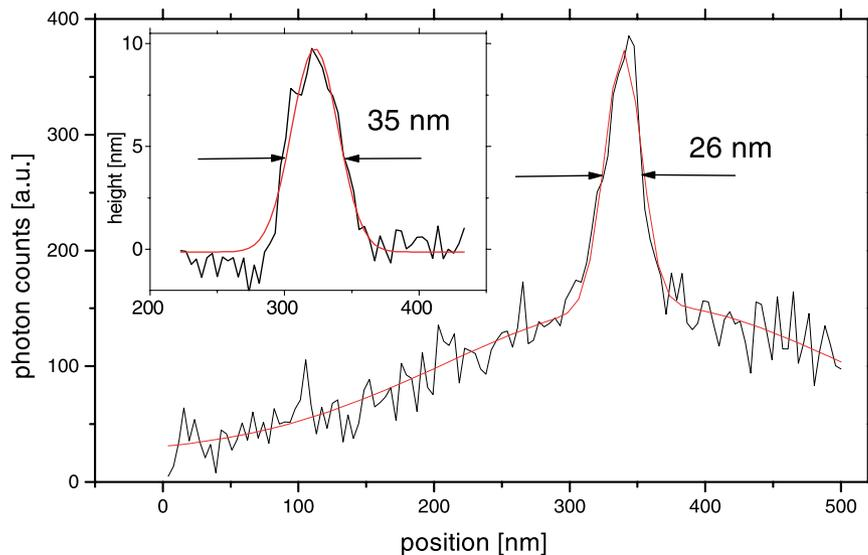
Fig. 7. Optical line scan of an isolated SWNT bundle integrating the intensity of the Raman band G'. The sharp near-field peak at  $\approx 330$  nm appears on top of a broad far-field contribution. (Red line) Fit curve consisting of two Gaussian peaks representing the near-field (FWHM = 26 nm) and far-field (FWHM = 330 nm) contribution. (Inset) Topography scan of the SWNT bundle indicating a height of  $\approx 10$  nm.
