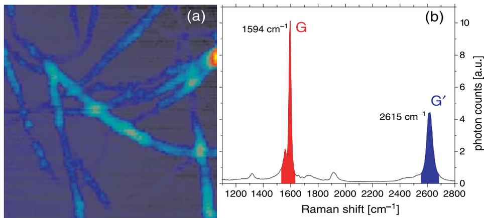
**Fig. 2.** (a) Topographic image of SWNT bundles on glass. Scan area  $1 \times 1 \mu\text{m}$ . Maximum height of the bundles is 30 nm. (b) Typical far-field Raman spectrum detected for bundles of SWNTs upon laser excitation at 633 nm. The characteristic Raman bands G (at  $1596 \text{ cm}^{-1}$ ) and G' (at  $2615 \text{ cm}^{-1}$ ) are marked to indicate the range used for spectral integration in Figs 4, 5, 6 and 7.
