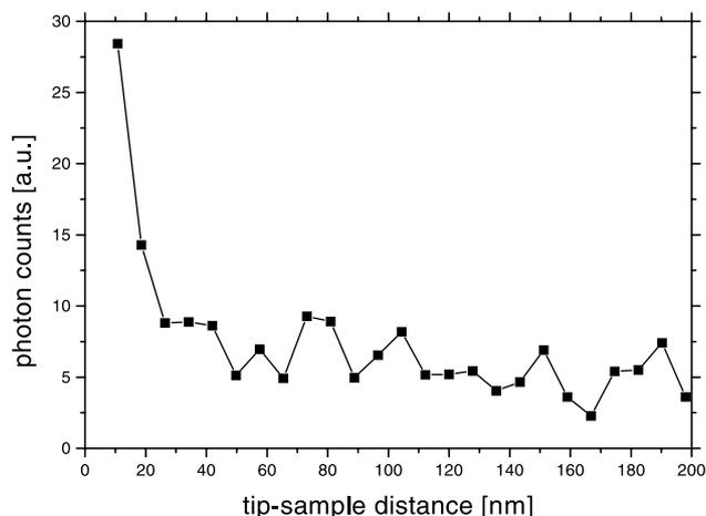
Fig. 6. Intensity of the Raman band  $G'$  of SWNTs as a function of the tip–sample distance. The steep increase for separations smaller than 20 nm indicates tip-enhanced Raman scattering in the near-field.
