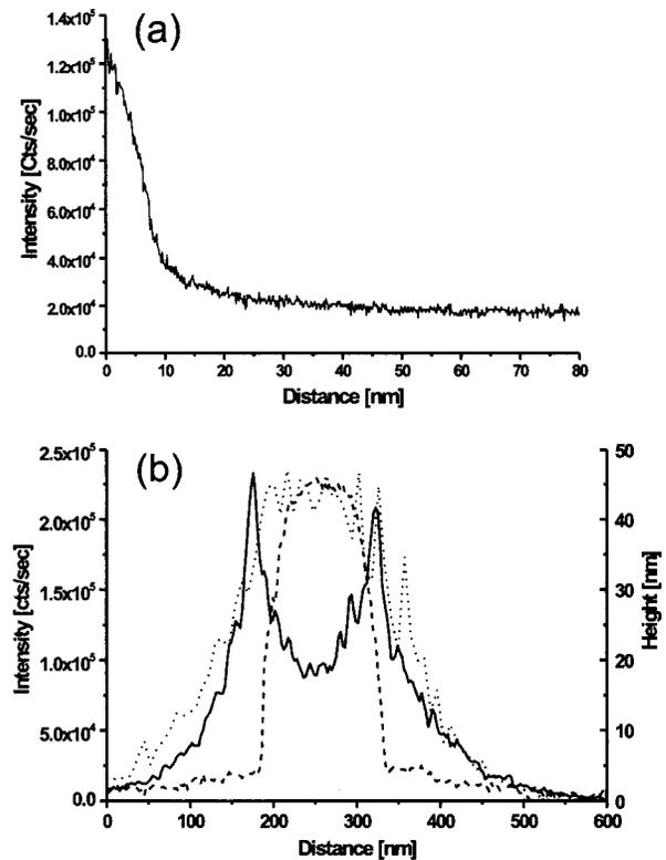
FIG. 3. (a) Photoluminescence decay on top of one of the field maxima shown in Fig. 2(a). (b) Cross section of the photoluminescence (solid curve), topography (dashed curve), and farfield photoluminescence (dotted curve). The luminescence enhancement is experienced within a nanometric volume of  $10 \times 10 \times 10 \text{ nm}^3$ .
