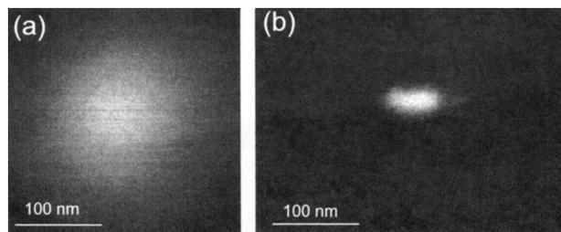
FIG. 1. (a) Two-photon photoluminescence image of a gold dimer scanned through the focal region of a 120 fs pulsed Gaussian beam. (b) Scanning electron micrograph of the dimer consisting of two 40 nm gold particles. The orientation of the dimer differs in the two images.
