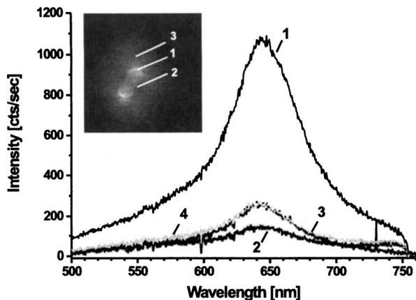
FIG. 4. Spectra of the dimer photoluminescence taken at different relative tip-dimer positions as indicated in the onset. The gray curve (4) represents the spectral response without the tip.
