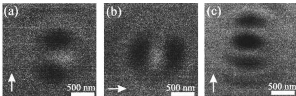
FIG. 4. Scan images recorded with a glass tip. A Gaussian excitation beam is used in (a) and (b), and a Hermite-Gaussian (1,0) beam mode is used in (c). The arrows indicate the direction of the incident polarization. A  $90^\circ$  polarization rotation leads to a rotation of the recorded pattern [(a) and (b)]. A contrast reversal is observed compared with Fig. 2. Images are  $2 \times 2\text{-}\mu\text{m}$  in size.
