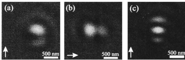
FIG. 2. Scan images recorded with a gold tip. A Gaussian excitation beam is used in (a) and (b), and a Hermite-Gaussian (1,0) beam mode is used in (c). The arrows indicate the direction of the incident polarization. A 90° polarization rotation leads to a rotation of the recorded pattern [(a) and (b)]. Images are  $2 \times 2\text{-}\mu\text{m}$  in size.
