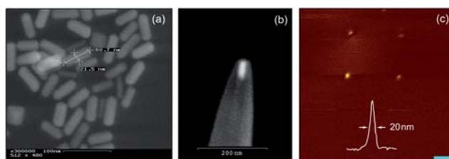
**Fig. 5** Optical half-wave antennas made of gold nanorods. (a) Colloidal synthesis of gold nanorods. (b) A single gold nanorod placed in the aperture of a nanoscale quartz pipette. (c) Near-field fluorescence image recorded with the optical half-wave antenna. The curve in the inset shows a cross-section through one of the fluorescence spots. Scale bar: 100nm.
