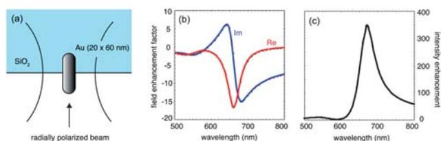
**Fig. 4** Electromagnetic calculations for a gold nanorod excited by a radially polarized beam and supported by a dielectric substrate. (a) Geometry used in the computations. (b) Real and imaginary parts of the field enhancement factor evaluated at the surface of the nanorod. (c) Corresponding intensity enhancement showing a resonance at  $\lambda \sim 650$  nm, red-shifted with respect to a spherical gold nanoparticle.
