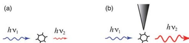
**Fig. 1** Enhancing the light-matter interaction with an optical antenna. (a) Incident radiation of frequency  $\nu_1$  gives rise to scattered radiation at frequency  $\nu_2$ . (b) An optical antenna improves the coupling between the radiation field and the molecule and enhances the intensity of the scattered radiation.
