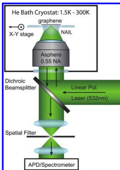
**Figure 1.** Schematic of the experimental setup. The sample was placed into a helium bath cryostat (1.55–300 K). The illumination and collection were accomplished through an aspheric lens combined with a NAIL that was bonded to the fused silica substrate. The signal was sent to either an APD or a spectrometer. An  $x$ - $y$  piezo scan-stage was used for confocal imaging and sample positioning.
