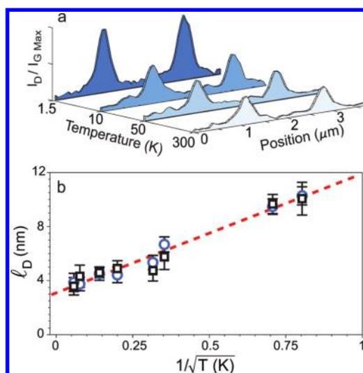
**Figure 5.** (a) Line scan profile for the ratio  $I_D/I_{G_{\text{Max}}}$  along the dashed line in Figure 2b evaluated for different temperatures. (b) Plot of  $l_D$  as a function of  $1/T^{1/2}$  for the left edge (blue circles) and the right edge (black squares) of the graphene sample. The dashed line shows a linear fit giving  $l_D \text{ (nm)} = 3 + 9/T^{1/2}$ .
