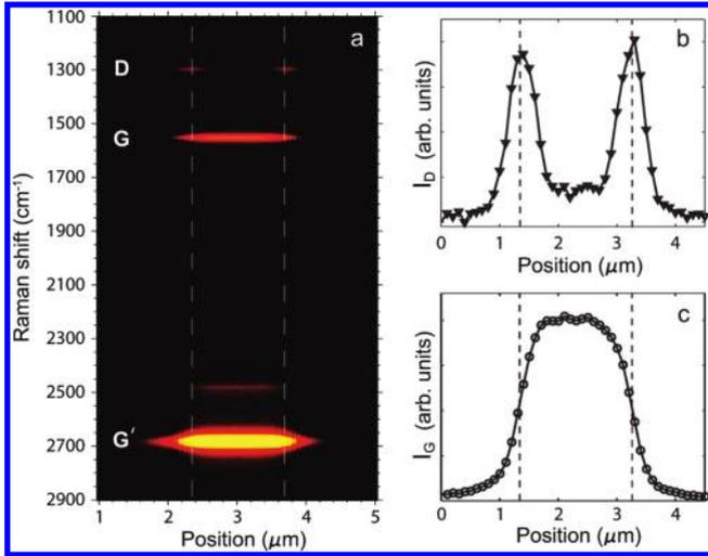
**Figure 3.** (a) Hyperspectral line scan recorded along the dashed line in panel b of Figure 2. The vertical lines indicate the position of the edges of the graphene piece. The D band is localized at the graphene edges. (b, c) Intensity profiles of the D and G bands obtained from the hyperspectral data shown in (a).
