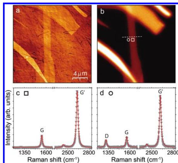
**Figure 2.** (a) Topographic image of exfoliated graphene deposited on a fused silica substrate. (b) Confocal Raman image showing the intensity of the G band over the same region. The dashed line indicates the direction along which Raman scattering spectra were recorded. (c, d) Raman spectra evaluated at the locations indicated by the square and circle in (b). The D band shows up only at the graphene edge. Spectrum d was scaled by a factor of 3 relative to spectrum c.
