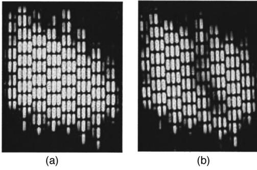
Fig. 3. (a) Photograph of a live CCD video image of a low-intensity interference pattern with which-way information encoded. (b) The same configuration but with a  $45^\circ$  analyzer after the polarimeter; note the single dark fringe through the center of the pattern.
