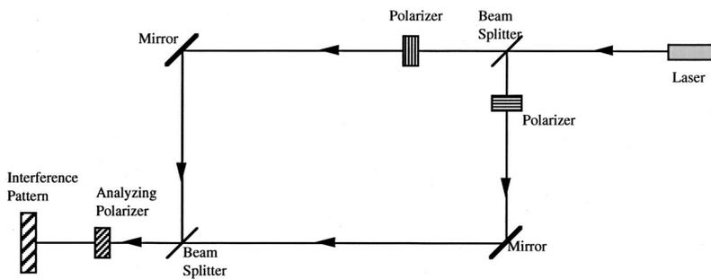
Fig. 1. Schematic view of the interferometer.
