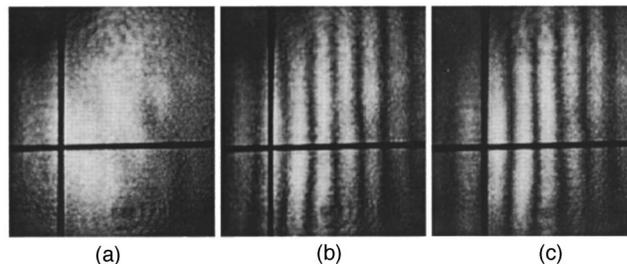
Fig. 2. Photographs of the interference patterns projected on a white screen. (a) The pattern resulting when which-way information is encoded in the polarization; (b) the pattern given after a final analysis by a  $45^\circ$  polarizer; (c) analyzed with a  $-45^\circ$  polarizer. The black cross is only to allow comparison of registration between figures. Note that (b) and (c) are complementary.
