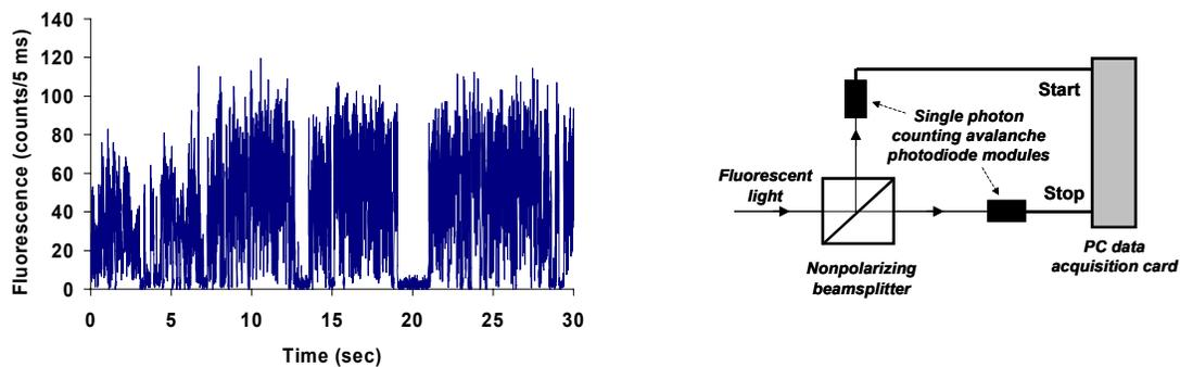
Figure 7. Left: Schematics of Hanbury Brown and Twiss setup for fluorescence antibunching measurements, right – changes of fluorescence intensity of single CdSeTe quantum dot in time (blinking).
