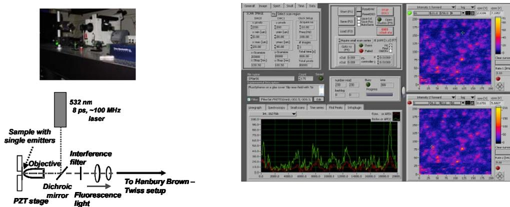
Figure 5. Left: Photograph and schematic of a home-built confocal microscope; right: User interface for single-emitter fluorescence imaging. Images of a raster scan of the sample show DiI-dye single-molecule fluorescence.
