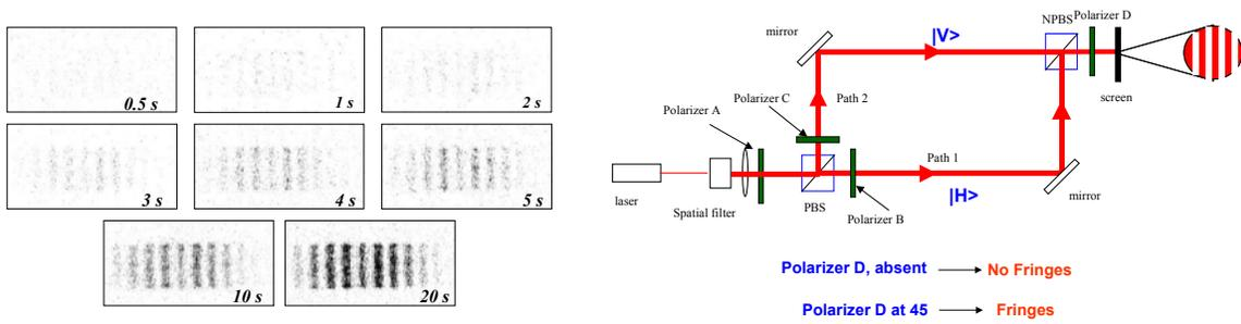
Figure 3, Left: Single-photon interference using Young's double-slit at different exposure time. Right: Mach-Zehnder interferometer schematics for "which-way experiment"
