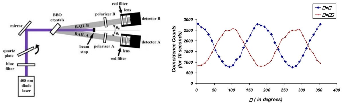
Figure 1. Left: Schematics of entanglement and Bell's inequalities experiment Right: Experimental polarization correlation's.
