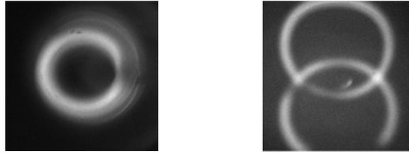
Figure 9. Example of student training results: spontaneous parametric down conversion cone of photons at the output of type I (left) and type II BBO crystals (right).
