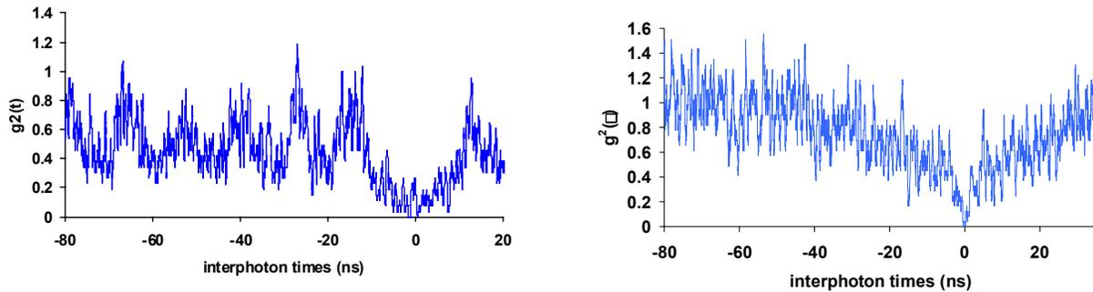
Figure 8, Left: Fluorescence antibunching of single PbSe quantum dot on bare glass slip under pulsed laser excitation (850 nm maximum fluorescence); right: fluorescence antibunching of single CdSeTe quantum dot in 1-D photonic bandgap cholesteric liquid crystal host (fluorescence lifetime of quantum dots is higher than the time interval between laser pulses).
