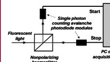
Fig. 4.1. Hanbury Brown and Twiss experimental setup for fluorescence antibunching measurements.
