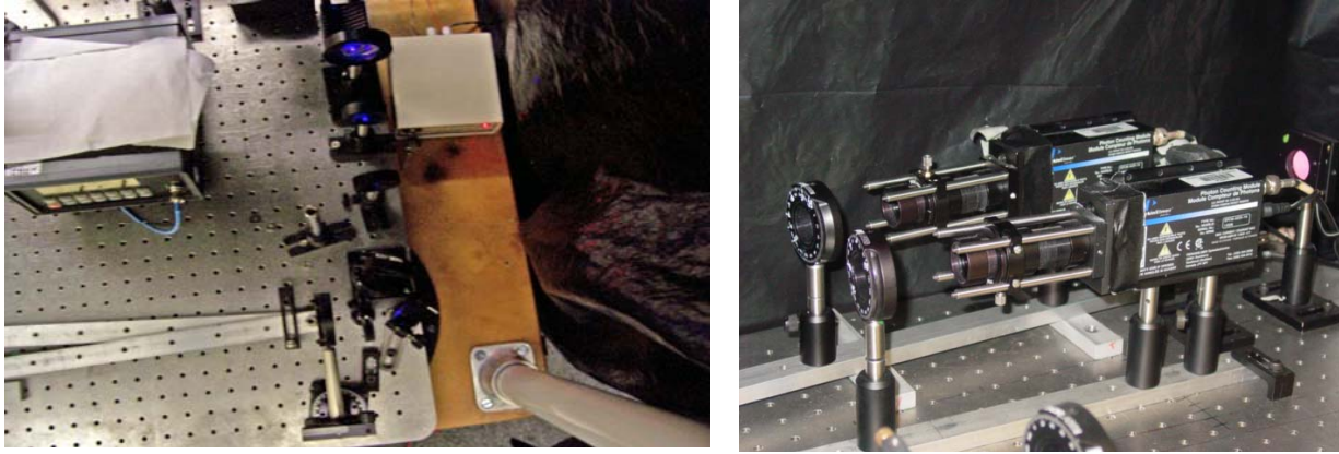
Figure 3. Part of entanglement lab setup with a diode laser excitation (left) (APDs and polarizers are not shown) and its entangled photon registration module with APDs and polarizers (right).
