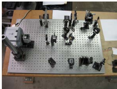
Figure 5. Photograph of single-photon interference setup with low-light level EM-CCD-camera (left); group of MCC students (right) carrying out this experiment.
