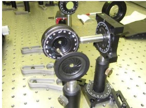
**Figure 2b. TOP: Photo of experimental setup. BOTTOM LEFT: Collection system with a 3-D adjustable mount with two polarizers and APD detectors. BOTTOM RIGHT: BBO crystal set with a 3-D rotation mounting (an iris diaphragm serves for alignment).**
