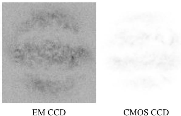
**Figure 10:** The intensity of the EMCCD image is much larger than the CMOS, but there is much less noise in the CMOS image, yielding better results. The inverse was taken of each image for clarity.
