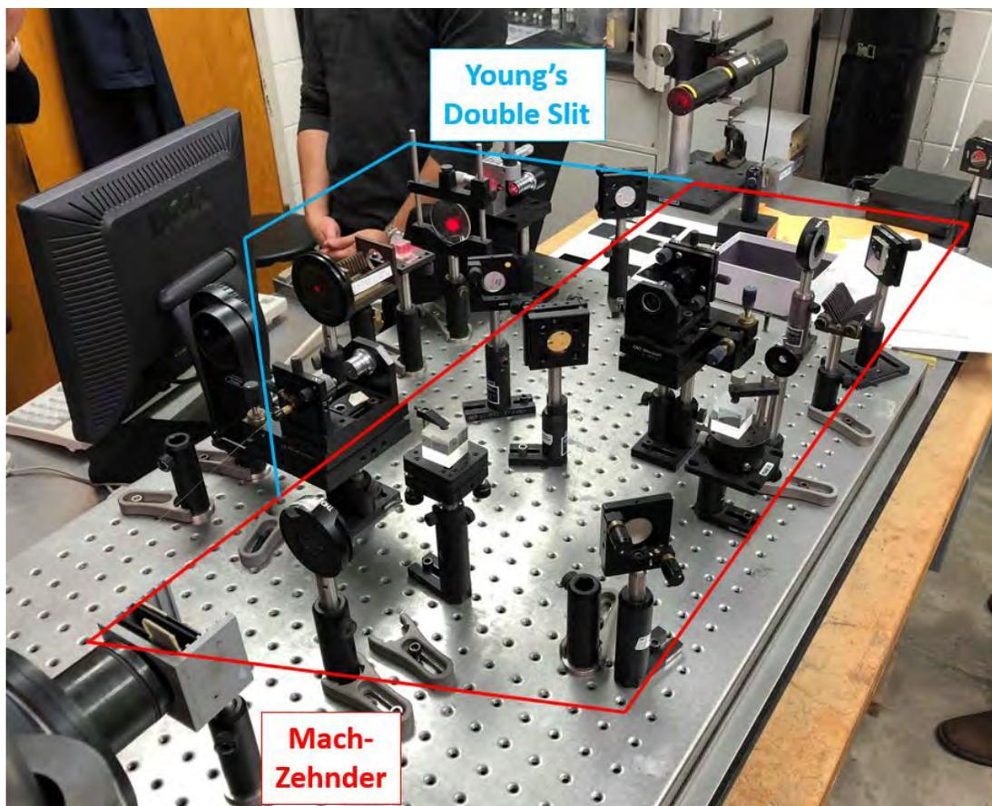
**Figure 3:** The lab setup of the two interferometers used.
