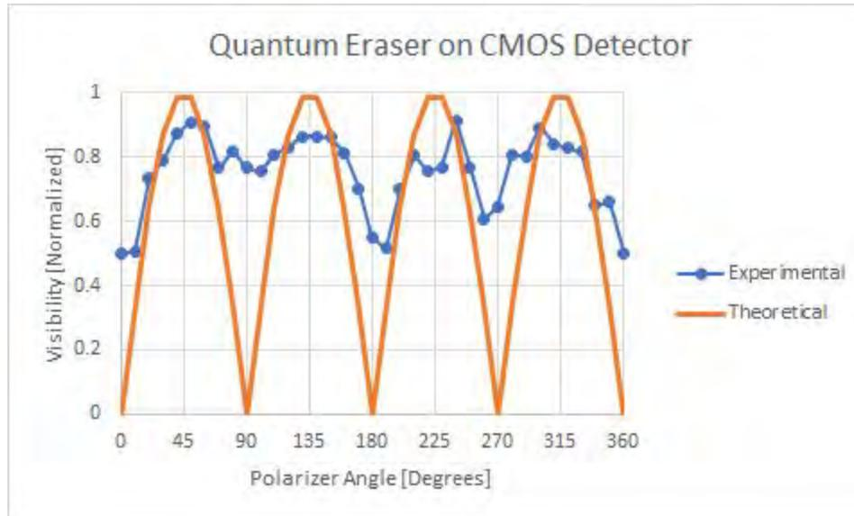
**Figure 12:** Visibility as a function of polarizer angle for the CMOS Detector.
