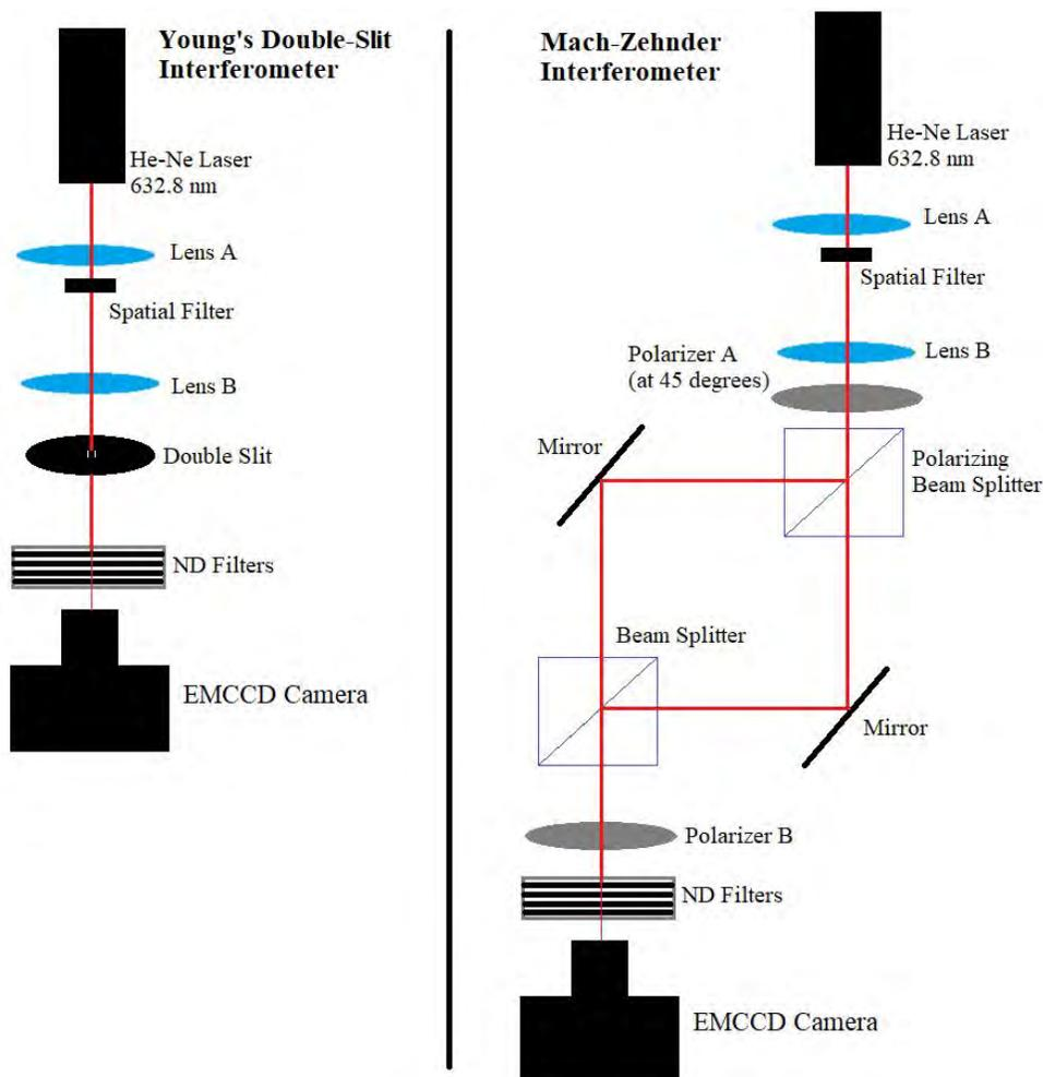
**Figure 2:** The experimental setup for the two types of interferometers. For the Mach-Zehnder interferometer Polarizer A is set to  $45^\circ$  in order to have an equal amounts of horizontally and vertically polarized photons that go through the polarizing beam splitter. After taking measurements on the EMCCD camera, we repeated the measurements with a CMOS camera.
