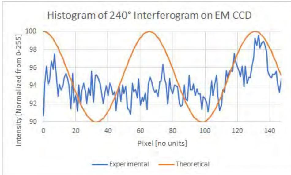
**Figure 7:** The histogram for one of the interferograms that has the highest fringe visibility. The noise distorts the results making it difficult to accurately calculate the visibility.
