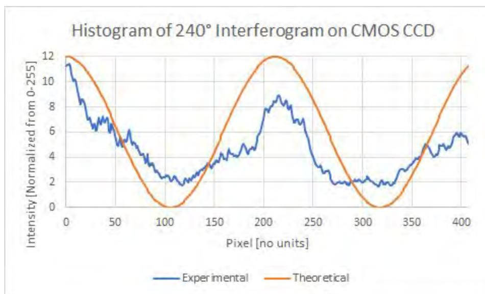
**Figure 11:** The histogram for the CMOS detector shows the interference pattern much better than that in figure 7. We used a 10s acquisition time for all of the images on the CMOS.
