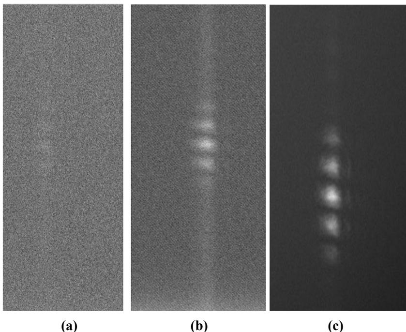
**Figure 5:** (a) 1ms acquisition time with no EM gain. You can barely start to see the fringes. (b) 1ms acquisition time with no EM gain and 20 accumulations. The fringes are very visible and there is less noise. (c) 20ms acquisition time, EM gain of 500, and 20 acquisitions. The fringes are extremely visible and you can start to see the second order fringes. The EM gain also gets rid of a lot of noise.
