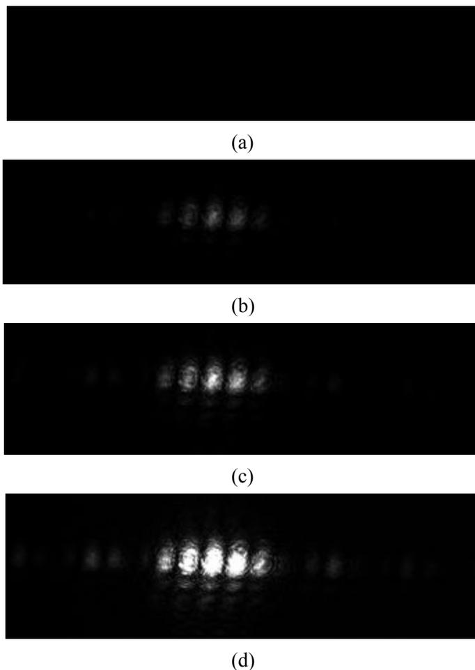
**Figure 9:** (a) 0.1s acquisition time. Fringes are not visible. (b) 1s acquisition time. Fringes are slightly visible. (c) 3s acquisition time. Fringes are clearly visible. (d) 10s acquisition time. Fringes are clearly visible and second order fringes are also visible.
