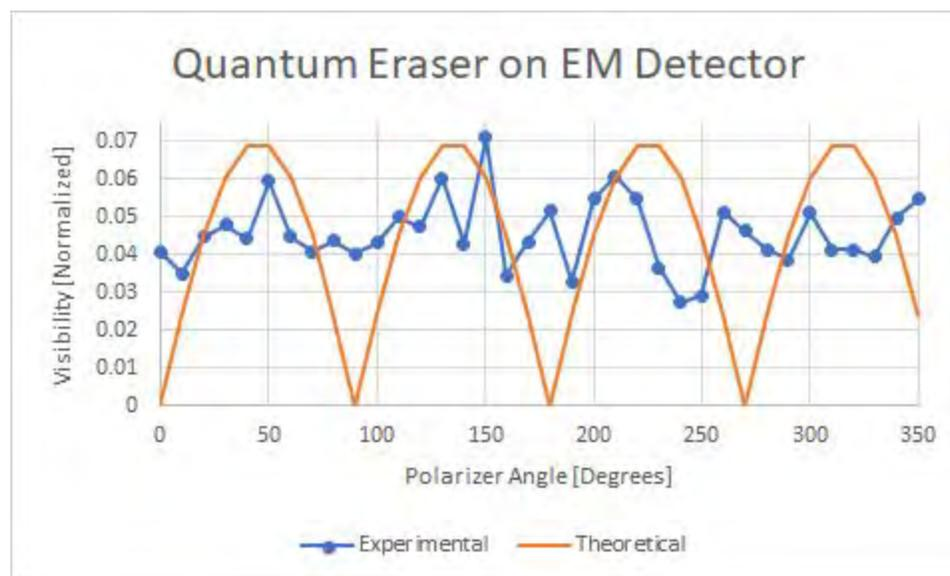
**Figure 8:** The visibility of the fringes for the EMCCD camera. The noise not only makes it difficult to see any pattern, but also lowers the amplitude to a fraction of the maximum visibility of one.
