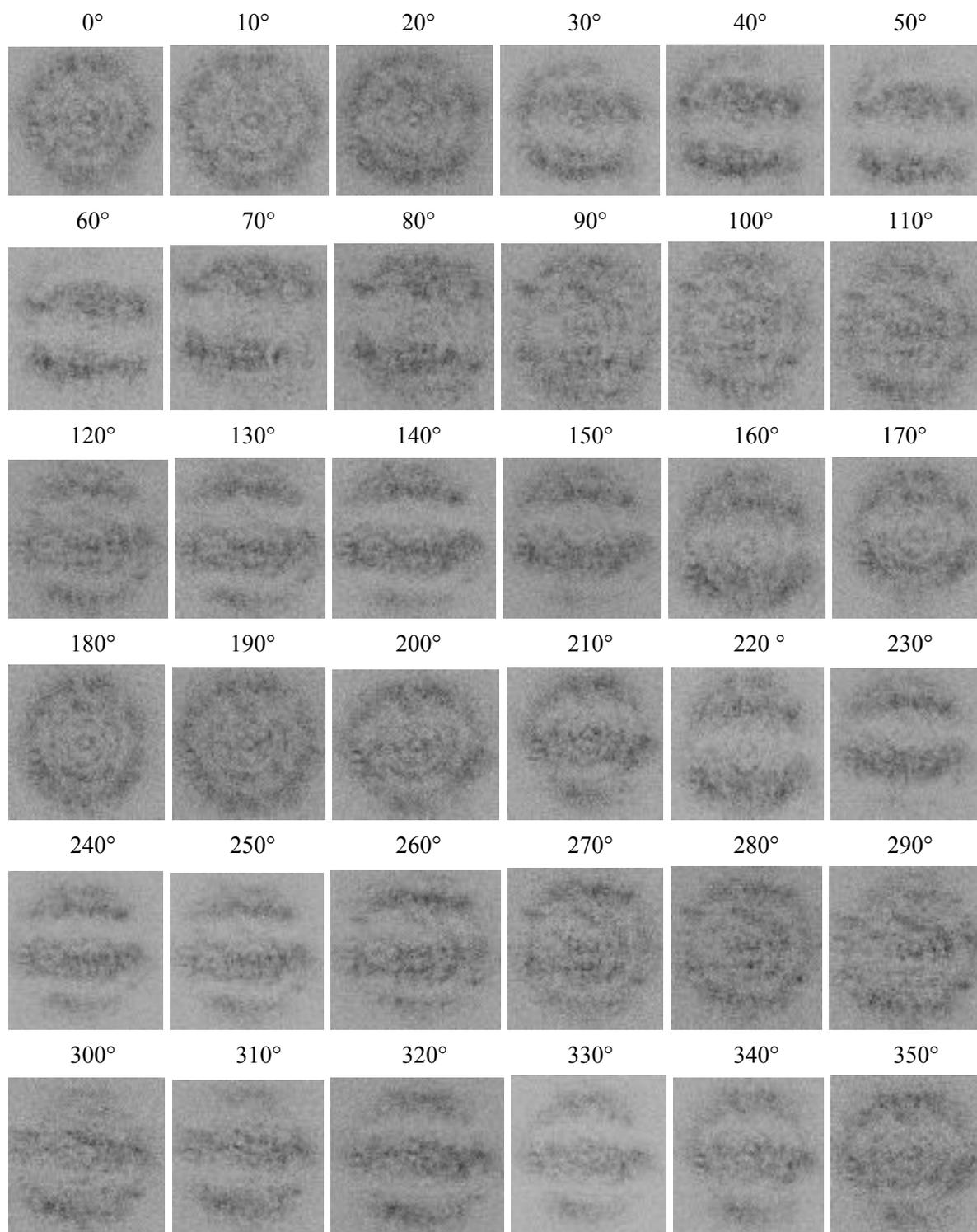
**Figure 6:** The interference pattern based on the polarizer angle with the images were inverted for clarity. We used no EM gain or accumulations and a 50ms acquisition time for each image.
