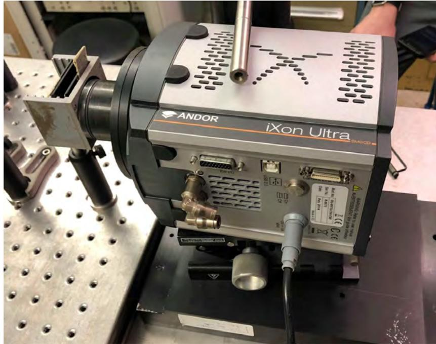
**Figure 4:** The EMCCD camera used in this lab.
