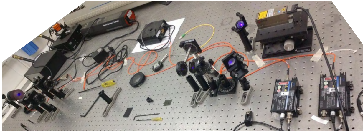
Figure 2.2: A photo of the actual lab setup used for Lab 1. Here, the 405 nm diode laser is on, and can be seen in the upper right. The beam is seen reflecting off the two alignment mirrors and entering the pair of BBO
