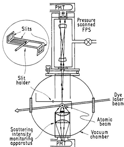
**Figure 1.** Experimental apparatus for AC Stark effect observation. The atomic beam is travelling out of the plane of the paper.
