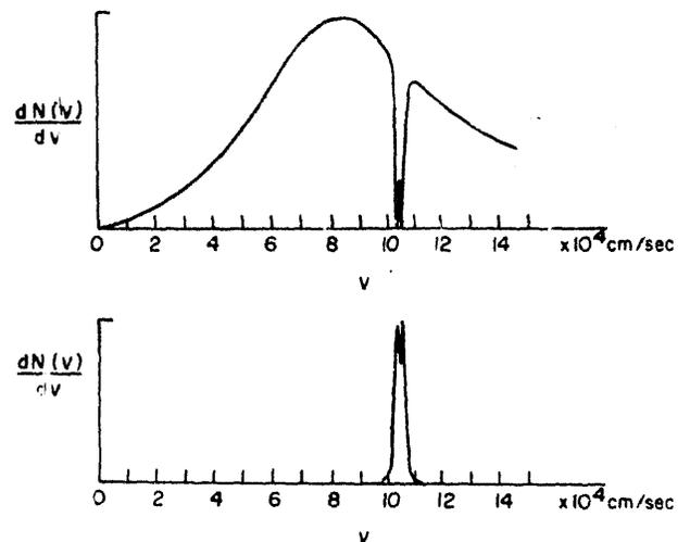
Fig. 3. (a) The velocity distribution of atoms in the  $F = 1$  ground state after pumping by laser beams 1 & 2. The hole is made up of two separate very closely spaced velocity components corresponding to the  $F = 1 \rightarrow 2$  &  $1 \rightarrow 1$  transitions. (b) The velocity distribution of atoms in the  $F = 2$  ground state after pumping. For the same reason, we again have two closely spaced components.
