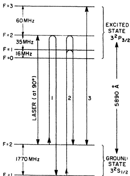
Fig. 1. Energy levels contributing to the Na  $D_2$  hyperfine structure. Note that the drawing is not to scale.
