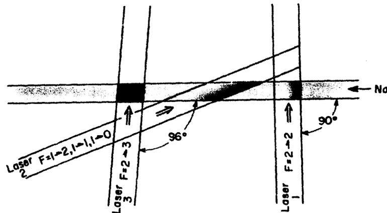
Fig. 2. Atomic beam – laser beam arrangement. All three laser beams are from the same laser reflected from appropriate mirrors. The shading in the region of intersection represents the fluorescence.
