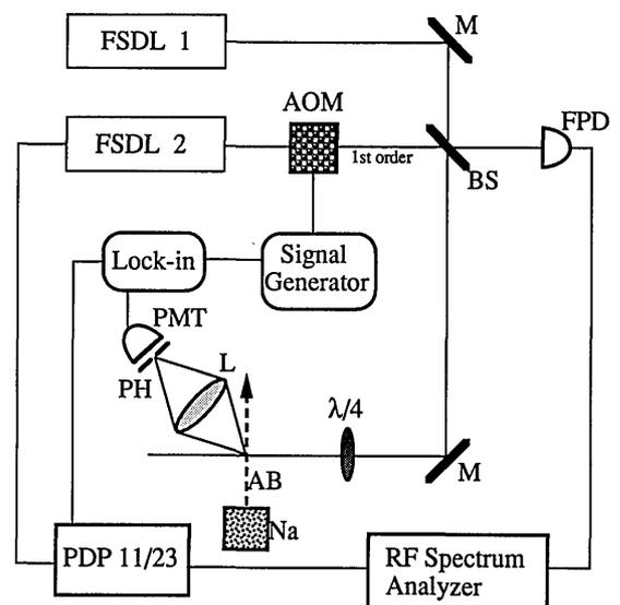
Fig. 2. Experimental apparatus. FSDL's, frequency stabilized dye lasers; AOM, acousto-optic modulator; M's, mirrors; BS, beam splitter; PH, pinhole;  $\lambda/4$ , quarter-wave plate; L, lens; AB, atomic beam; PMT, photomultiplier tube; FPD, fast photodiode; PDP 11/23, microcomputer.
