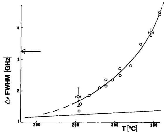
Fig. 4. Measured linewidths versus temperature. The bottom line is the normal Doppler linewidth. The arrow shows the linewidth expected from process (1). Typical error bars are given. The laser was tuned to the  $D_2$  line and fluorescence was at 8195 Å.
