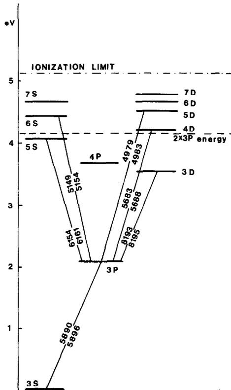
Fig. 1. Level diagram of Na.
