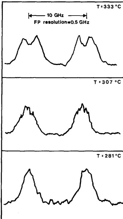
Fig. 3. Typical traces of lineshapes. The Fabry-Perot free spectral range is 10 GHz and the resolution is better than 1 GHz. The laser was tuned to the  $D_2$  line, and the fluorescence was at 8183 Å.
