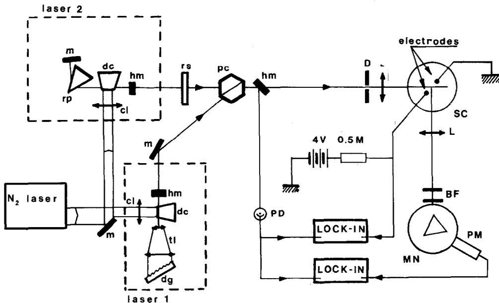
Fig. 5. Experimental set-up. cl = cylindrical lens, dc = dye cell, dg = diffraction grating, hm = high transmission mirror, m = 0% transmission mirror, pc = Glan prism, rp = rutile prism, rs = polarization rotator, BF = interference filters, D = diaphragm, L = lens, PD = trigger photodiode, PM = photomultiplier, SC = sodium cell.
