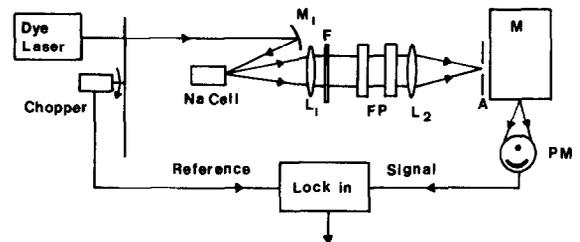
Fig. 2. Experimental set-up. The dye laser is cw with a ring cavity producing up to 100 mW with a bandwidth of 1 GHz.  $M_1$  is a mirror with focal length of 20 cm,  $L_1$  and  $L_2$  are lenses with focal lengths of 15 cm, F is an RG-10 Schott filter, FP is a Tropel model 360 tunable Fabry-Perot interferometer, A is a pinhole aperture, M is a 82410 Jarrel-Ash monochromator. PM is an EMI 9659A extended S20 photomultiplier and lock-in is a PAR 128 lock-in amplifier.
