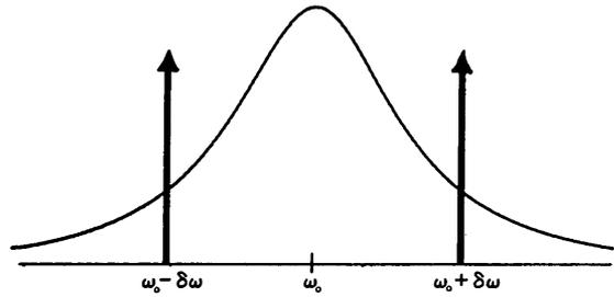
Fig. 3. The assumed bichromatic operating state of the laser. The total laser field is made up of two strong-field components of equal amplitude that are symmetrically displaced from the gain center.
