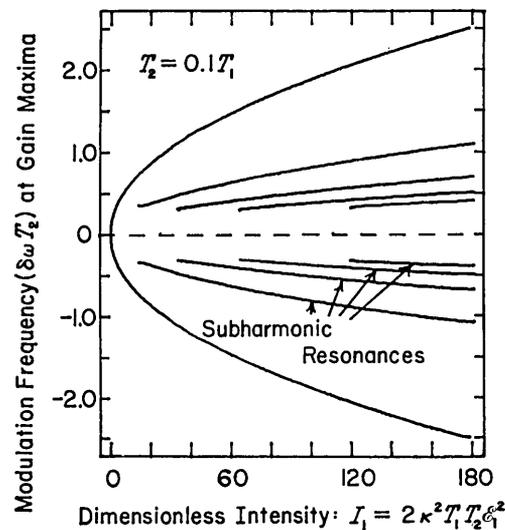
Fig. 6. Location of maxima in the gain profile as a function of intensity. The outer curve is a parabola that corresponds to modulation at the Rabi frequency. The other curves are portions of parabolas that correspond to modulation at subharmonics of the Rabi frequency. The particular intensity at which each of the subharmonic resonances first appears is determined by the relaxation times of the gain medium.
