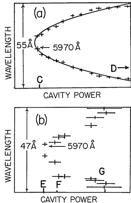
Fig. 2. Spectral output of the dye laser as a function of cavity power. (a) The pairs of operation frequencies on the C, D branch have a parabolic dependence on the cavity power. (b) The pairs of operation frequencies on the E-G branch appear to fall on another parabola.
