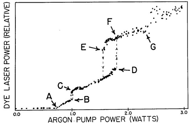
Fig. 1. Experimentally measured dependence of intracavity power on the argon-pump power. Letters indicate the various thresholds of instability; see corresponding points in Fig. 2. Single-frequency operation occurs only between points A (lasing threshold) and B.
