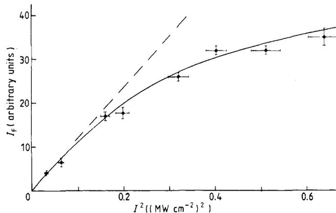
**Figure 2.** The atomic saturation characteristic for counterpropagating two-photon absorption where  $\gamma_D = 0$  and  $\gamma_L = 0.34$  GHz. The integrated fluorescent intensity ( $I_F$ ) is plotted against the square of the laser peak pulse focused intensity ( $I^2$ ).
