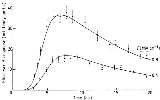
**Figure 4.** The theoretical and experimental time development for two-photon absorption for  $\gamma_D = 0$  and  $\gamma_L = 0.34$  GHz. The intensity indicated against the curve is equal to  $\sqrt{I_1 I_2}$ .
