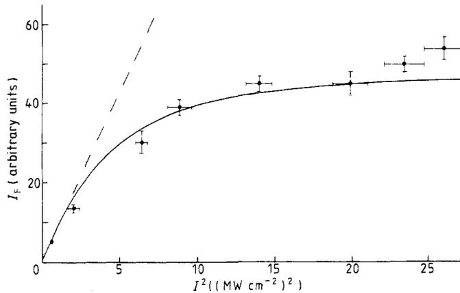
**Figure 1.** The atomic saturation characteristic for copropagating two-photon absorption where  $\gamma_D = 3.38$  GHz and  $\gamma_L = 3.60$  GHz. The integrated fluorescent intensity ( $I_F$ ) is plotted against the square of the laser peak pulse focused intensity ( $I^2$ ).
