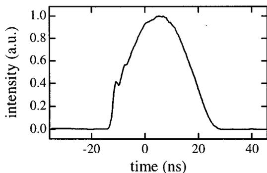
FIG. 8. Temporal profile of a single-longitudinal-mode dye laser when pumped by a single-mode (smooth) pump laser. The rapid rising edge is indicative of the output from the low- $Q$  dye cavity.
