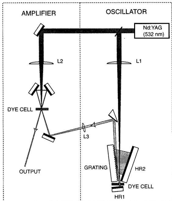
FIG. 1. Schematic layout of the oscillator and amplifier system. L1 is a 250 mm focal length lens and L2 is a 150 mm focal length lens. HR1 and HR2 are high reflectivity mirrors.
