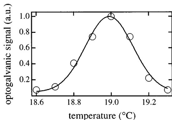
FIG. 3. Optogalvanic signal as a function of temperature of the dye fluid (open circles). The best fit Gaussian (Doppler) profile is shown as the solid line.
