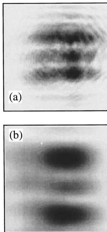
FIG. 5. Spatial profiles of the pump and dye lasers showing the impact of gain guiding in the oscillator. In (a) is the Nd:YAG mode incident on the dye cell. In (b) is the resultant dye beam.
