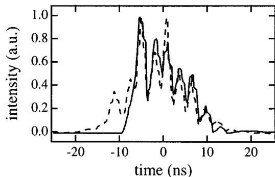
FIG. 7. Temporal profile of a single-longitudinal-mode dye laser (solid line) when pumped by a multilongitudinal mode Nd:YAG laser. Shown as a dashed line is the pump temporal profile [from Fig. 2(a)] that produced the dye laser pulse. The temporal structure in the dye laser pulse follows that of the pump.
