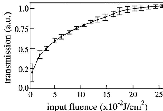
FIG. 9. Normalized transmission of the dye beam as a function of the input dye fluence. The transmission is normalized to the saturated value because the measurement did not account for the reflection losses in the cell. A smooth line is drawn through the data points with error bars indicating the noise standard deviation.
