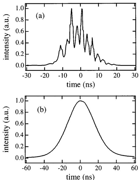
FIG. 2. Temporal profile of the Nd:YAG pump laser. In (a), the laser is actively  $Q$  switched and is multilongitudinal mode, and in (b) the laser is passively  $Q$  switched and is single-longitudinal mode.
