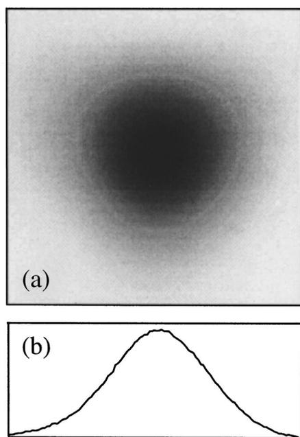
FIG. 4. (a) Spatial profile of the dye laser. (b) Cross section of the profile taken horizontally through the center of the beam showing its near Gaussian spatial quality.
