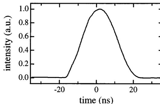
FIG. 10. Temporal profile of the single-mode dye laser beam after saturable absorption in the dye amplifier.
