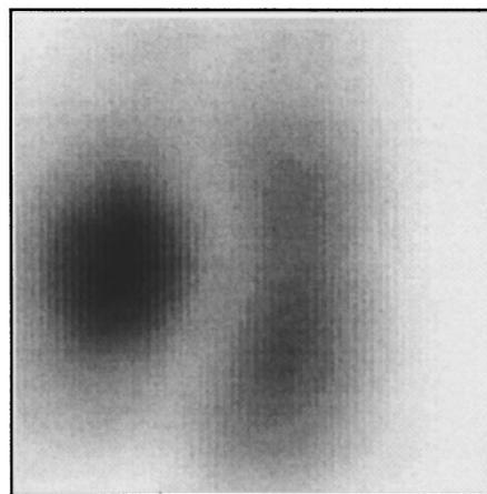
FIG. 6. Spatial profile of the dye beam in a quasisingle-longitudinal-mode laser. The two lobes are present when the laser is running in two longitudinal modes.
