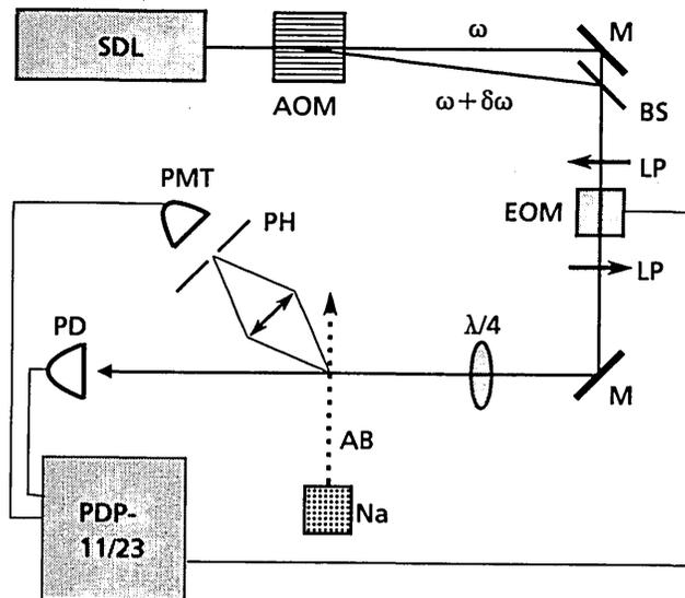
Fig. 4. Experimental apparatus: SDL, stabilized dye laser; AOM, acousto-optic modulator; M's, mirrors; BS, beam splitter; LP's, linear polarizers; EOM, electro-optic modulator;  $\lambda/4$ , quarter-wave plate; Na, sodium oven; AB, atomic beam; PH, pinhole; PMT, photomultiplier tube; PD, photodiode.
