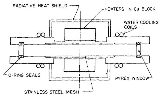
Fig. 1. Cross-sectional view of the disk-shaped heat-pipe oven.
