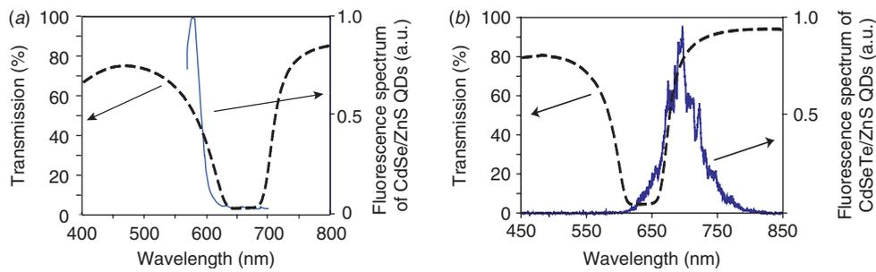
Figure 2. Selective transmission of two monomeric chiral photonic bandgap CLC hosts for right-handed circular polarized light and the fluorescence spectrum of the CdSe (a) and CdSeTe (b) QDs. (The color version of this figure is included in the online version of the journal.)
