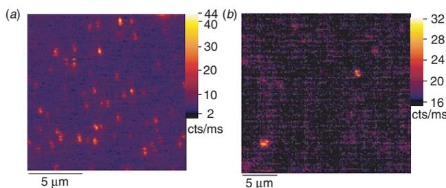
Figure 4. Typical confocal fluorescence images (1) of single CdSe QDs in CLC host (a) ( $15\mu\text{m} \times 15\mu\text{m}$  scan), and single PbSe QDs in CLC host ( $25\mu\text{m} \times 25\mu\text{m}$  scan) (b). (The color version of this figure is included in the online version of the journal.)
