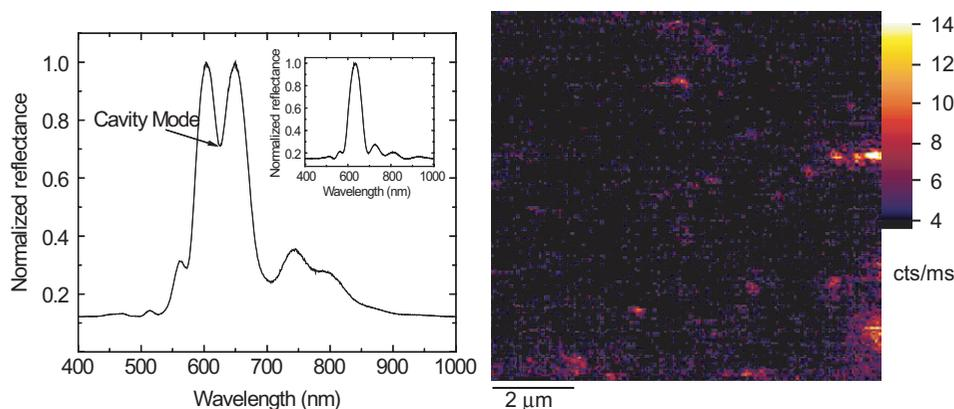
Figure 7. (a) Reflectivity spectrum of the polymeric microcavity embedded with CdSe QDs with  $\lambda_0 = 620$  nm. Shown in the inset is the normalized reflectivity spectrum showing the stop band of the ten-period Bragg reflector without the defect layer. (b) Single QD fluorescence imaging in a polymeric microcavity under 532-nm excitation ( $10 \mu\text{m} \times 10 \mu\text{m}$  scan). (The color version of this figure is included in the online version of the journal.)
