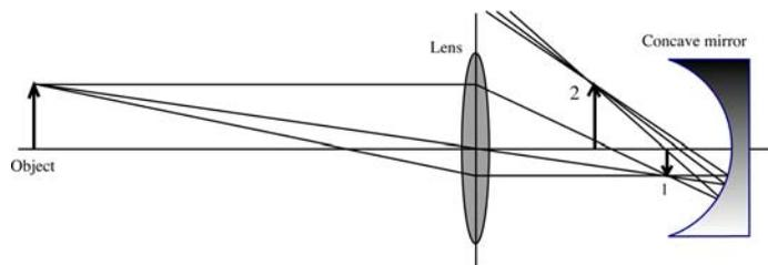
Fig. 1. Della Porta's 1589 projection system, producing an upright image at 2.
